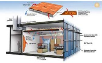
As a restaurant heats up during the day and cools off at night, ESP's thermal energy storage solution acts like a sponge, absorbing and releasing energy that can be used to moderate the temperature. The result is a passive process that can deliver a 20% reduction on HVAC operating cost .
